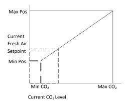
The highest value between free cooling demand output and interpolation output for the fresh air setpoint will be the output to the fresh air damper.
