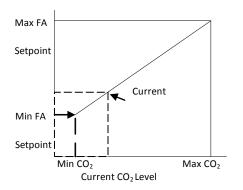
The highest value between free cooling demand output and interpolation output for the fresh air setpoint based on the CO2 level will be the output to the fresh air damper
